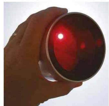
▲ The etalon is the heart of many solar scopes
